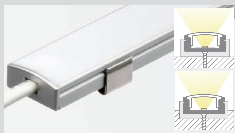
P01B Aluminum profile with white PMMA lens for surface or recessed installation with limited width. Equipped with angle-joint accessory.
