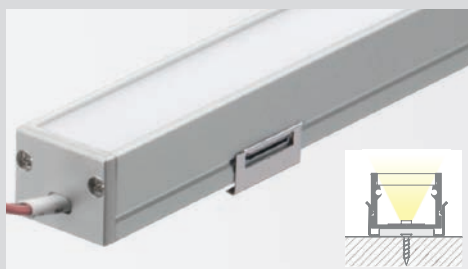
P03B Aluminum profile with polycarbonate lens with uniform light distribution for surface or recessed with suitable clips.
