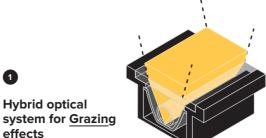
The <u>Grazing optic</u> is perfect for enhancing and highlighting a texture. To optimize the effect, the fixtures must be installed near the surface that is being lit (0.13in), close together or in a continuous line.
