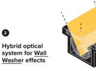
The <u>Wall Washer optic</u> allows uniform and consistent lighting of wide surfaces. The ideal distance (a) of Jedi wall washers from the wall should be around one fourth of the surface height (h) - Arrangement: a= 1/4 x h. By installing the fixtures at a distance of about 79in (fixture center) and at 47in from the wall, it is possible to obtain a uniformly illuminated surface with an average of 14 foot candles.
