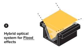
The <u>Flood optic</u> is ideal for lighting moldings on a façade with a soft lighting effect. On the plane transversal to the fixture it features a relatively narrow emission that makes it possible to not waste light outside the surface to be lit. On the plane parallel to the fixture, the emission is wide yet controlled to focus on specific elements.
