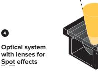
The <u>Spot optic</u> provides a more concentrated and vertical emission, perfect for highlighting architectural elements. The precise and narrow beam is controlled for reducing lateral spillage along the length of the fixture making Jedi the ideal professional solution for projected light.
