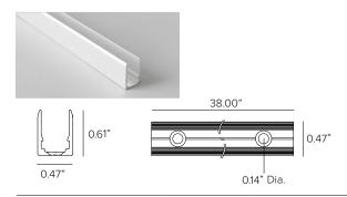
DURAFLEX ARCH SIDE aluminum rigid profile with 2ea screws. Note, termination end prep rest to outside of the profile.
