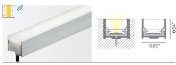
Aluminum high impact walk over rated profile with frosted polycarbonate lens for recessed installation. Dimension: 118"L (3M). Profile must be shipped via freight only. For efficient shipping via UPS/FedEx, lengths can be cut to 59" upon request.
