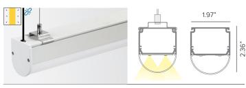
Aluminum profile with domed 180° opal polycarbonate lens for suspension installation. Dimension: 118°L (3M). *Profile must be shipped via freight only. For efficient shipping via UPS/FedEx, lengths can be cut to 59° upon request.*
