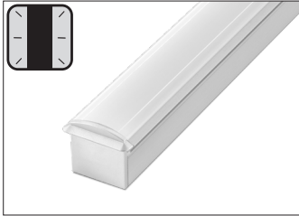
PRIN-U Flush mount aluminum profile. Anodized aluminum rigid profile complete with opal translucent diffuser cover. Available in 79in (2M) lengths.
