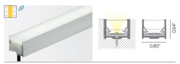
Aluminum high impact walk over rated profile with frosted polycarbonate lens for recessed installation. Dimension: 118"L (3M). **Profile must be shipped via freight only. For efficient shipping via UPS/FedEx, lengths can be cut to 59" upon request.**
