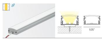
Aluminum profile with opal polycarbonate lens for surface or recessed with suitable clips. Dimension: 118"L (3M). **Profile must be shipped via freight only. For efficient shipping via UPS/FedEx, lengths can be cut to 59" upon request.**
