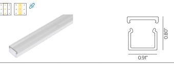
Two-piece PVC mounting tube; white opaque base with cover (clear or frosted). Countersink screw holes, 12" O.C. Dimension: 96"L
