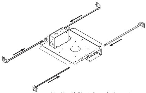
Use Non IC Plasterframe for low wattage fixtures and in cases where there is not any contact with insulation
