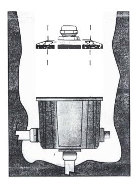
Connect brass box to conduit system. Seal conduit entries inside junction box with a good grade RTV sealant after sealant manufacturer's instructions.
