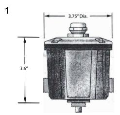
The brass box is supplied with the following components: 4 3/4"Side/Bottom NPT holes. 4 1/2" reduction NPT adapters
