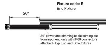
10 ft power cord and dimming lead cables with IP68 connectors attached onto each cable (provided with Solo fixtures)
