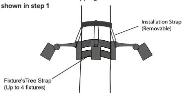
Once Tree strap is secured with the fixture's tree strap belt secured below, assemble and connect the line voltage box with the fixtures and power up the connection box with 120VAC power only
