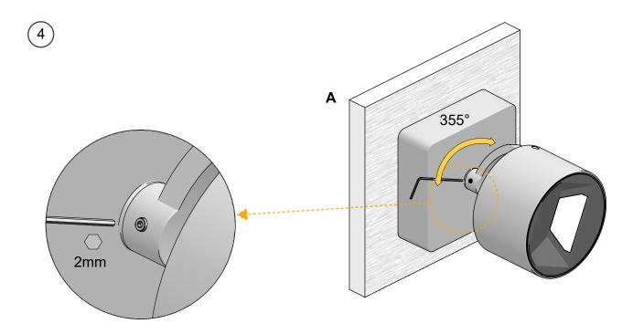
The optical unit can be adjusted 355° on the horizontal plane with aiming locking system.
