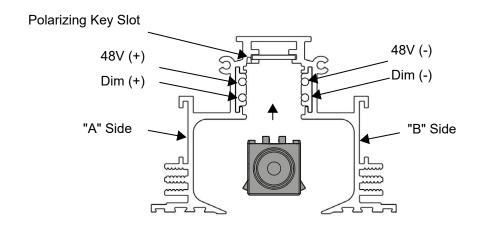
\*Track is shipping with "A" and "B" Labeling for correct Polarity.
