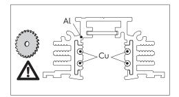
**MULTISYSTEM Evo Track can be** field cut to required length with use of a Chop saw and appropriate saw blade for cutting Aluminum.
