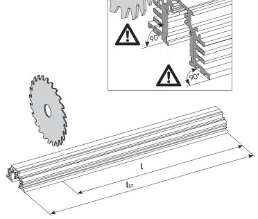
After cutting track to length, trim off Conductor Rails to
