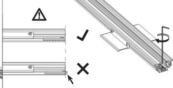
Joint Connector should align to end first track.
