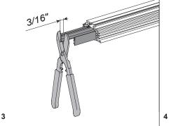
After cutting Conductor Rails, insert back into tracks.
