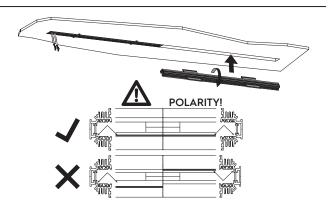
Insert next track into ceiling with correct porarity direction.
