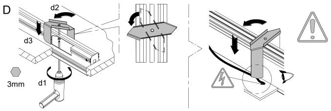
Once profile has been inserted, adjust brackets by turning them counterclockwise to secure profile on ceiling or walls
