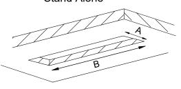
The installer will need to cut an aperture on the ceiling or wall where the profile and power rails will be installed depending on the profile specified
