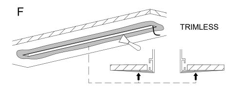
The finishing of the ceiling and or walls can begin after profile has been secured, simply apply drywall mud compound and paint.
