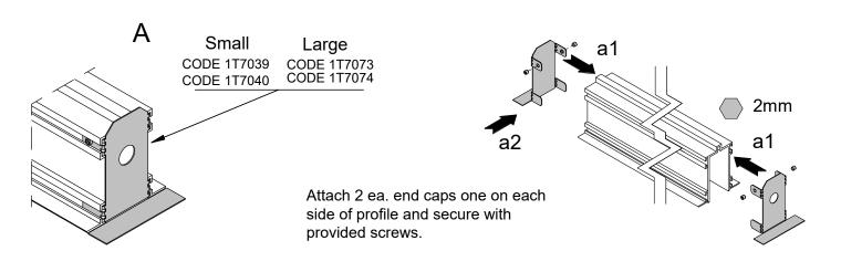
Attach mounting clips on back side of profile and secure with provided screws (do not tighten the screws) В
