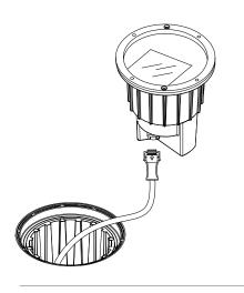
Connect female IP68 DSMT lead cable connector onto fixture's connector, make sure both locking wings are on lock position before inserting the fixture into the mounting sleeve.
