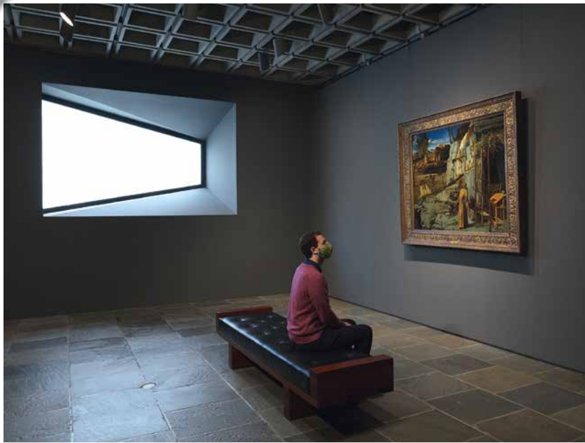
⌄ The gallery's irregular window is equipped with a fritted light-reducing, UV-blocking film, while a single fixture is equipped with a filter to subtly shift from 3000K to a cooler 3400K to blend with natural daylight.
