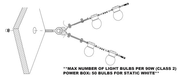
WIRING DIAGRAM STATIC WHITE
