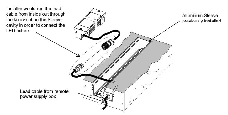
Secured by tightening the lock ring turning it to "close" direction to ensure a sealed connection.
