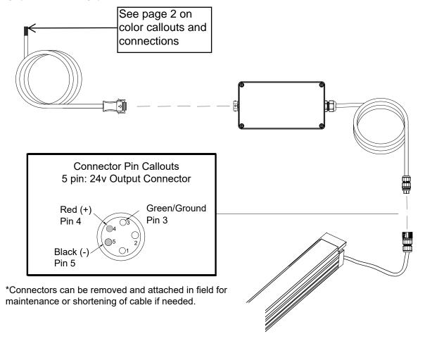
Secured by tightening the lock ring turning it to "close" direction to ensure a sealed connection.
