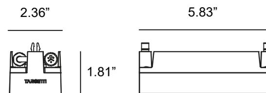
IVY wireless Bluetooth Casambi power feed and dimming control box, for individual fixture control
