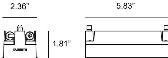
IVY 0-10V power feed and dimming control box, for group fixture control.
