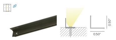
Aluminum L-Profile 1/2" x 1/2" for linear run lengths. Duratape can be mounted at either 0° or 90° mounting positions. Countersink screw holes, 12" O.C. Dimension: 96"L.
