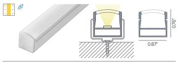
Surface mount anodized aluminum rigid profile complete with opal translucent lens. Dimension: 79"L (2M)
