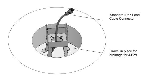
Stainless Steel base with rods for concrete pouring \*Refer to mounting base installations instructions
