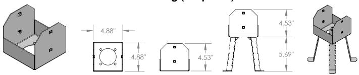
Trimless mounting base with ground anchor fixing rods for installation in concrete. AISI 316 stainless steel. Mounting bolts included. **Required for use with 1US2530 by NEC.**
