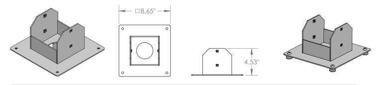
Powder coated mounting plate for surface installation outside the post. AISI 316 stainless steel compatible with dowels to be inserted into 4 holes, Ø 0.34" Dia. for use with 5/16" bolts maximum. Anchor bolts not included. **Required for use with 1US2530 by NEC.**
