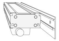
JEDI flush mount bracket with countersink screw holes for attachment.
