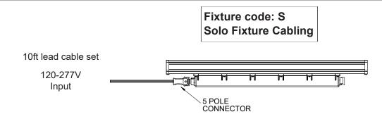
Solo - 10ft EPDM JACKET 16-6 lead cable with DSM&T connector and additional DSM&T cap for dead end.
