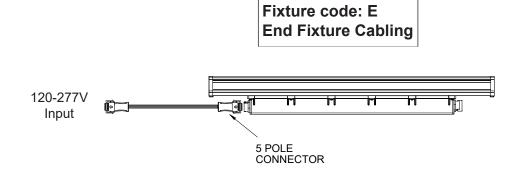
**End** - 32" EPDM JACKET jumper cable with DSM&T connectors and additional DSM&T cap for dead end.
