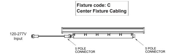
Center- 32" EPDM JACKET 16-6 jumper cable with DSM&T connectors.
