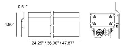
JEDI anodized aluminum anti-glare side cover mounts with a slight standoff to eliminate glare for direct view applications. Side cover option allows for a fluid finished appearance that can be field painted to match the architectural finish.
