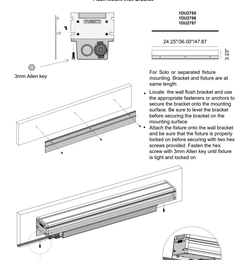
For inner connected fixtures mounting, set seams of flush mount bracket to stagger seams of fixtures.
