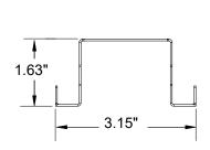
JEDI end cap, 1ea. Kit include 1ea 1E2754 Bracket to mount at end of fixture. Used to create finished end for side cover mounting applications.
