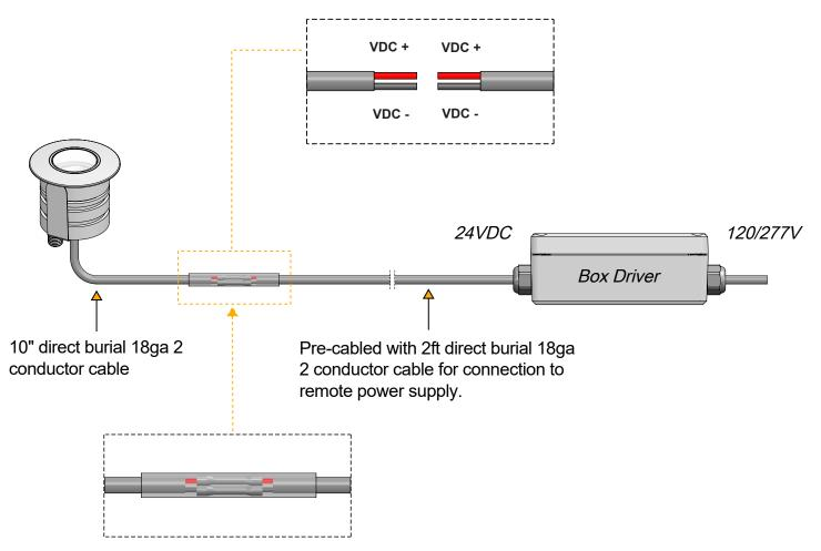
Waterproof Heat-shrink solder seal connectors and Heat-shrink tube (included with fixture)
