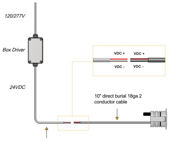
Pre-cabled with 2ft direct burial 18ga 2 conductor cable for connection to remote power supply.
