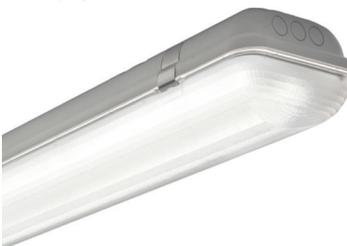
Concentrated elliptical distribution. Internal high efficiency specular aluminum reflector with clear diffuser in self-extinguishing V2 polycarbonate, photo-engraved interior, UV stabilized, injection molded with smooth outer surface. Available for 50" and 61.92" fixture lengths only.
