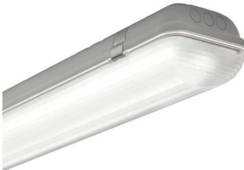
Internal high efficiency specular aluminum with clear diffuser in self-extinguishing V2 polycarbonate, photo-engraved interior, UV stabilized, injection molded with smooth outer surface. Available for 50" and 61.92" fixture lengths only.
