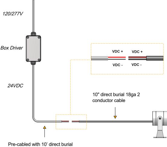
Pre-cabled with 10' direct burial 18ga 2 conductor cable for connection to remote power supply
