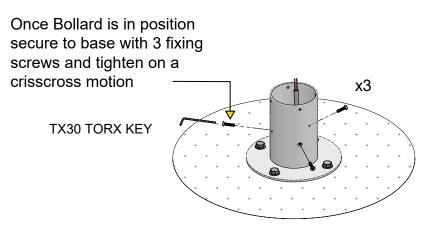
**Step 3.** Connect 25ft pre-cable into fixture's head with connector Butt 22-18 AWG. Once a secure connection has been made, insert fixture head into Bollard and rotate to desired illumination direction.
