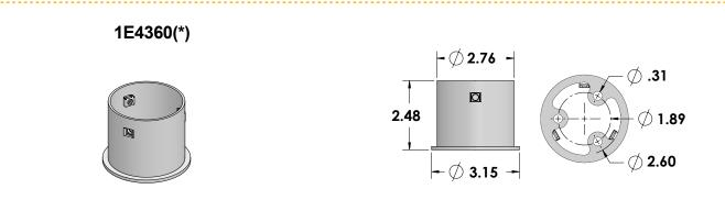
Trimless surface mounting base. Powder coated AISI 316 stainless steel.
